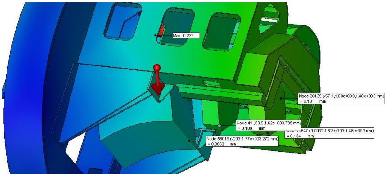
135 degrees magnet displacement (Maximum magnet displacement is 0.134 mm < 0.3mm)
