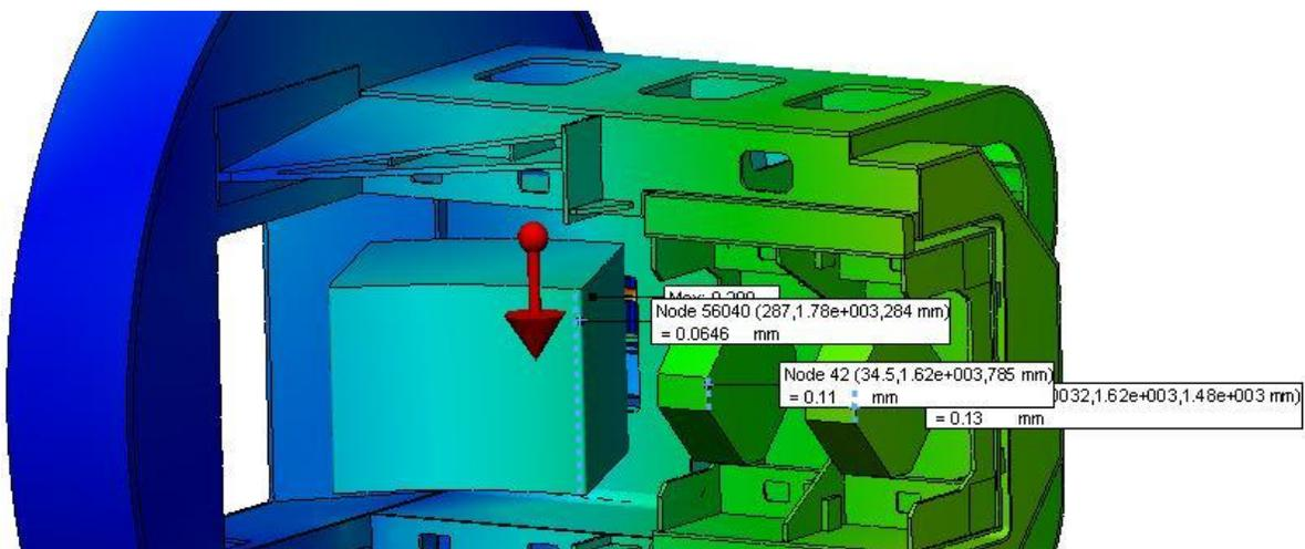
90 degrees magnet displacement (Maximum magnet displacement is 0.13 mm < 0.3mm)
