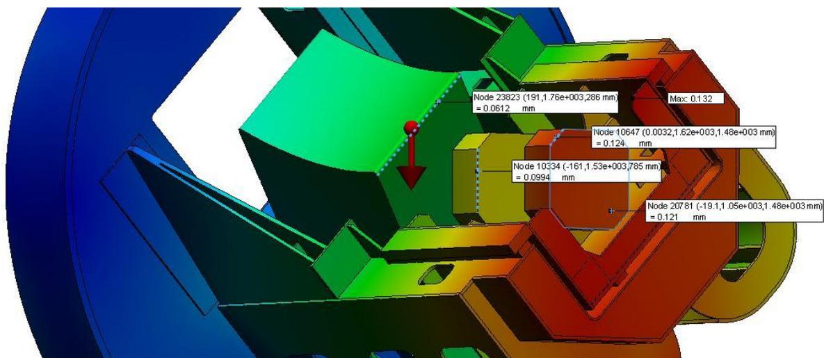
45 degrees magnet displacement (Maximum magnet displacement is 0.124 mm < 0.3mm)
