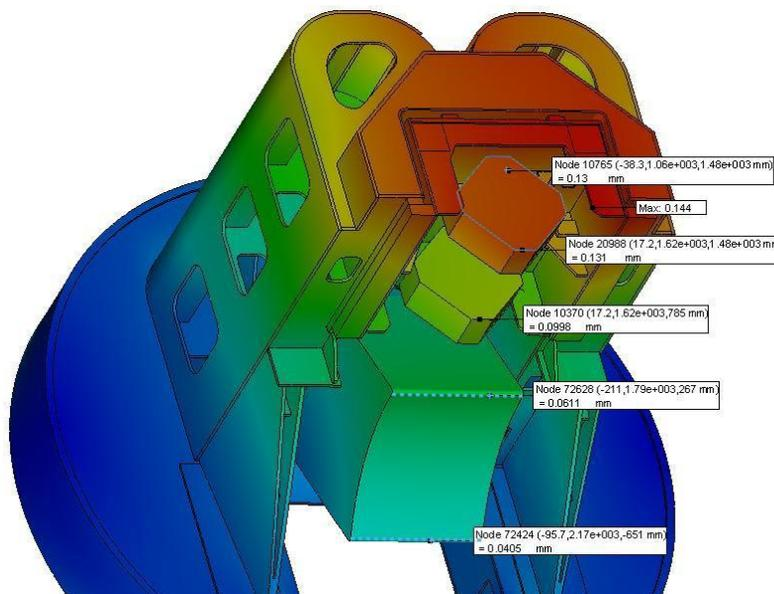
180 degrees magnet displacement (Maximum magnet displacement is 0.131 mm < 0.3mm)
