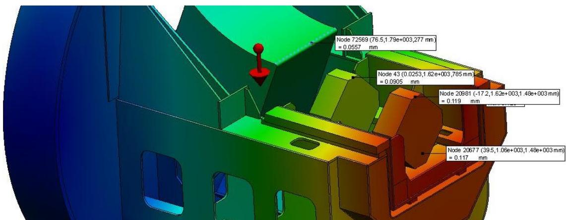
0 degrees magnet displacement (Maximum magnet displacement is 0.119 mm < 0.3mm)
