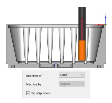
Tool path can be generated from Top to Bottom or Bottom to Top
