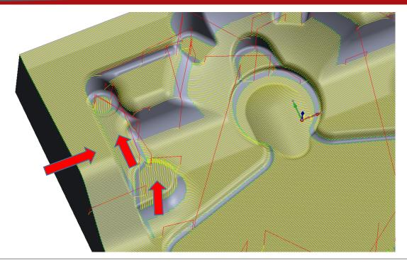
Automatic optimal angle of machining in XY-plane
