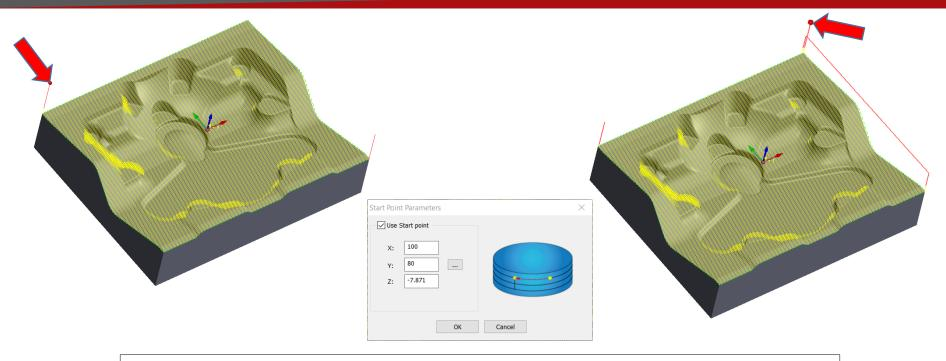
User can change the start point of the tool path by picking a vertex or a predefined point from which the tool should start machining
