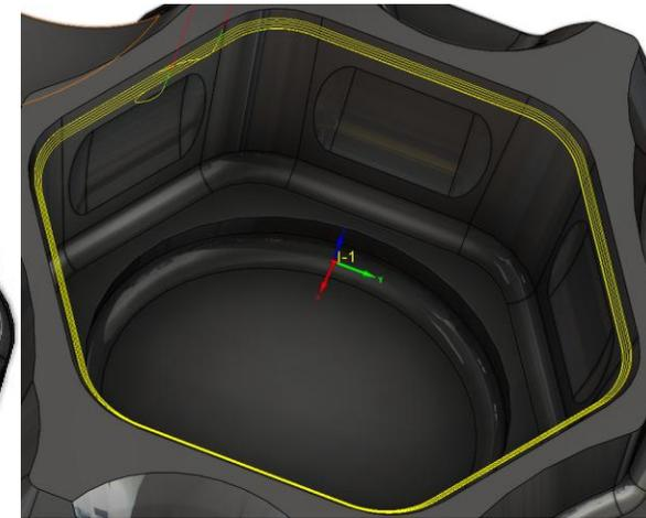
**Spiral Cutting Method:** Enables multiple cuts using a spiral pattern on closed contours, avoiding stepover marks on chamfered or radius edges, providing a smoother toolpath with fewer machine movements.
