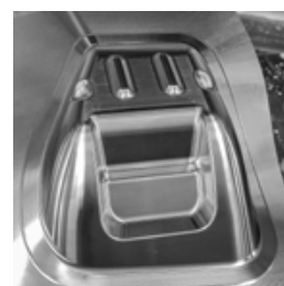
Excellent surface finish of 0.4 \mu\text{m} with SolidCAM HSM strategies
