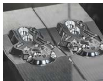
Excellent surface finish of 0.4 \mu\text{m} with SolidCAM HSM strategies
