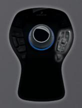
The key to SpaceMouse Pro's smooth and intuitive 3D navigation is the patented six-degrees-of-freedom (6DoF) sensor.
