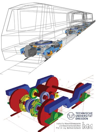
**SIMPACK Rail** is an add-on module tailored to the specific requirements of the rail sector and is the world-wide market leader for rail vehicles multi-body simulation. SIMPACK Rail is used to simulate the dynamics of all rail vehicles or complete trains.
