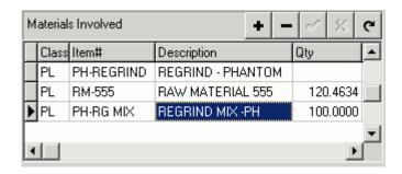
The system would use the 100 lbs of the regrind mix on hand and because there was not any regrind it would consume the rest in the virgin raw material component (RM-555) to equal the 220.463 lbs required.
